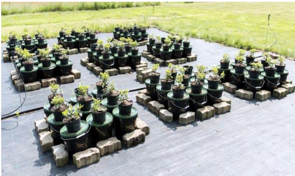
Image 1. The experimental set-up a) the leachate collection devices (LCDs) constructed from 10L plastic buckets intercepted all leachate draining through the 2l containers of Viburnum tinus 'French White' and b) The lay out of the Mypex plot, plants were blocked in randomised groups of nine.
